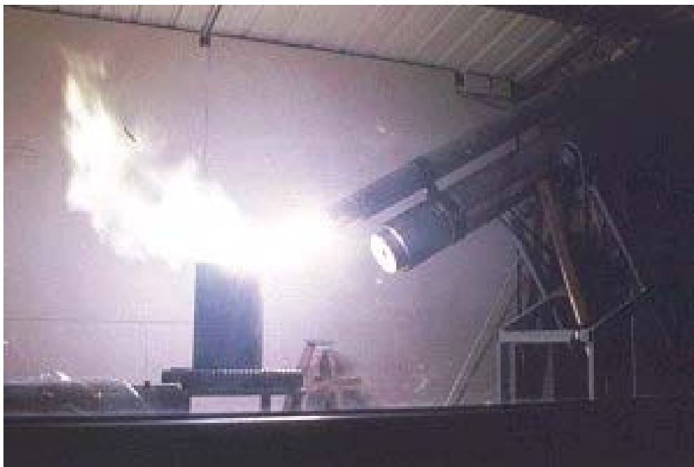
Figure 3-8. Plasma Arc Torch Operating (Source: http://www.zeusgroup.org/applications.html ).
